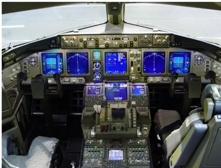
Figure 6.31: The cockpit of the Boeing 777. Note that most flight information is displayed on several computer operated displays.
