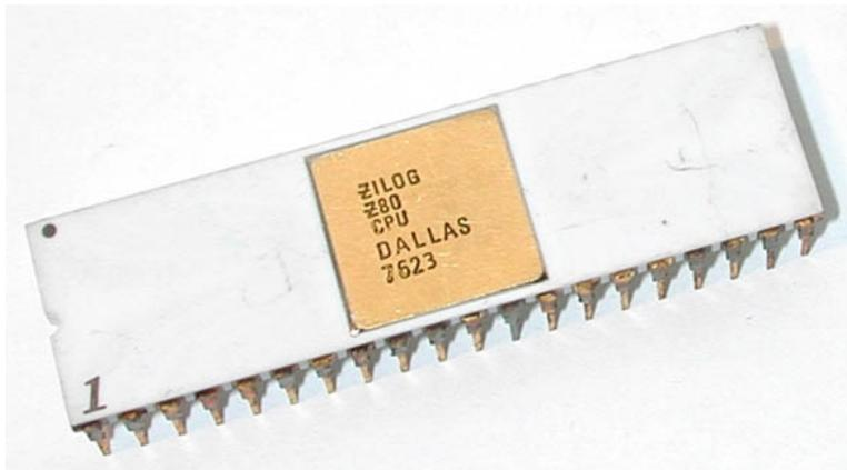
Figure 6.28: A Zilog Z80 microprocessor manufactured in 1976.
