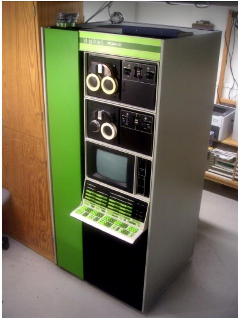
Figure 6.27: A PDP-12 minicomputer manufactured by Digital Equipment Corporation about 1970.
