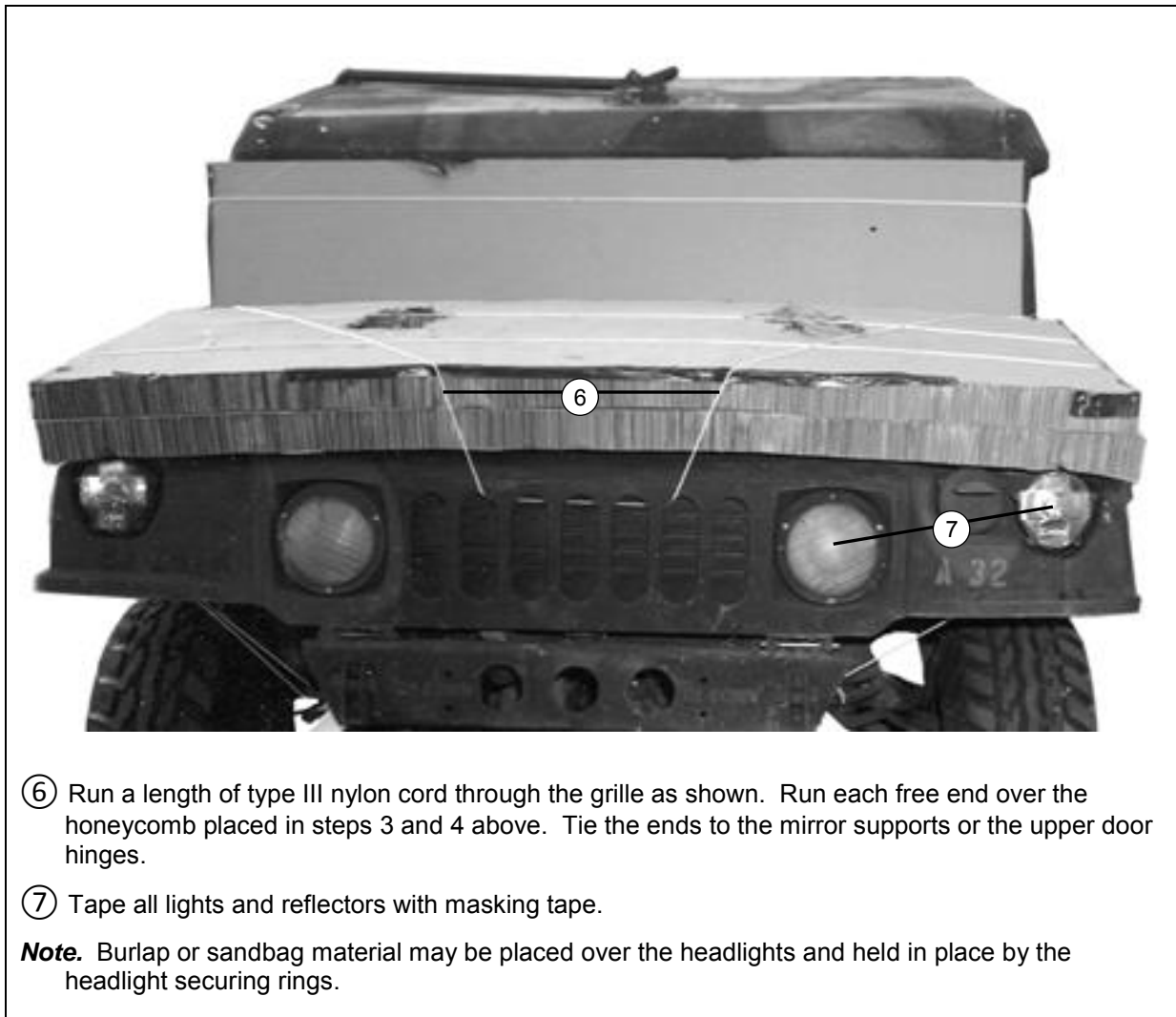
Figure 7-11. Honeycomb Placed on Front of Ambulance and Mirrors Folded (continued)
