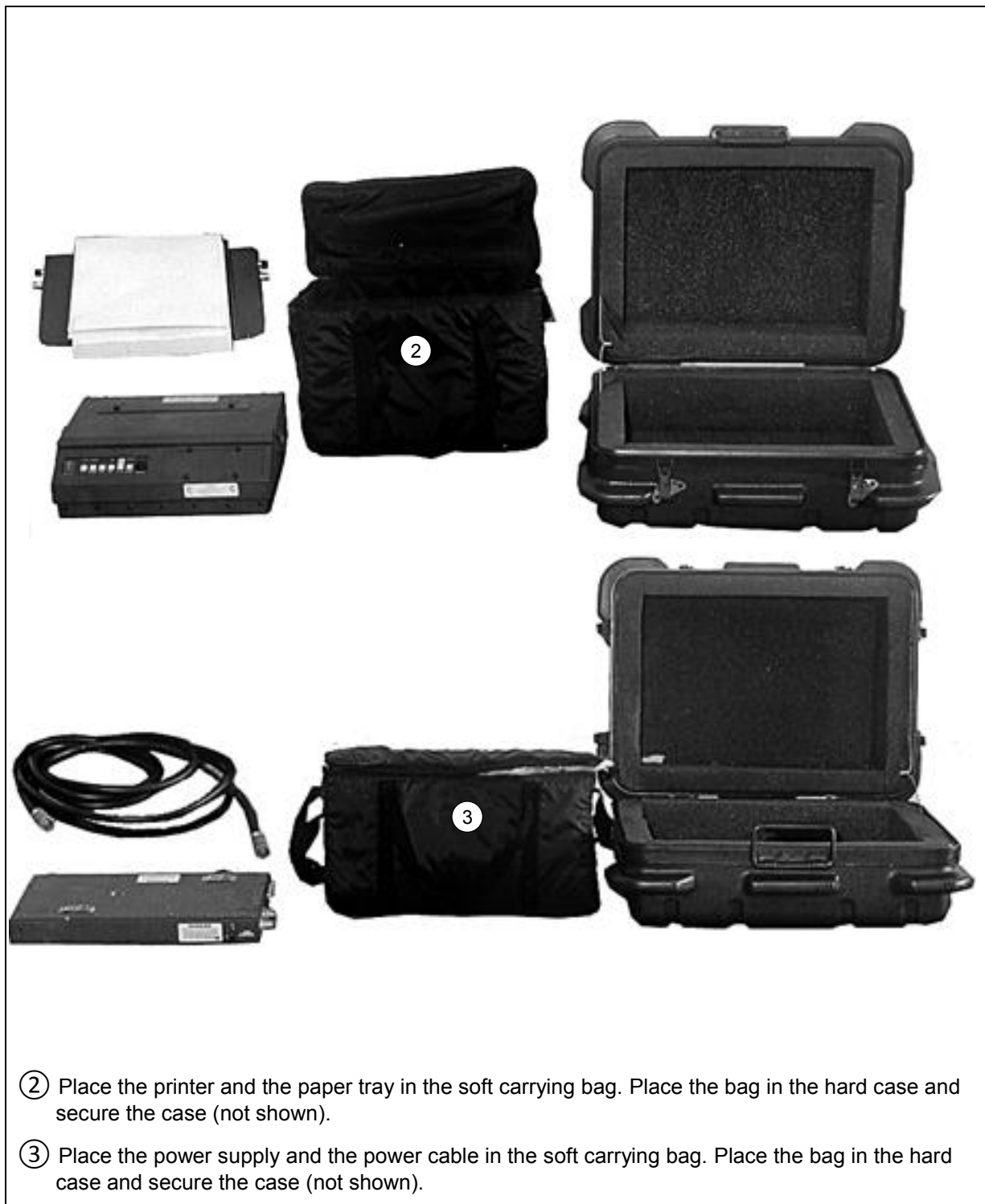
Figure 4-22. Initial Fire Support Automated System Rigged in M998 Truck (continued)
