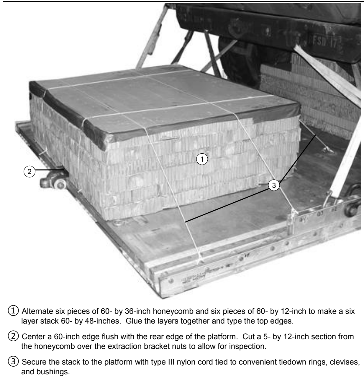
Figure 7-24. Parachute Stowage Platform Prepared and Installed
