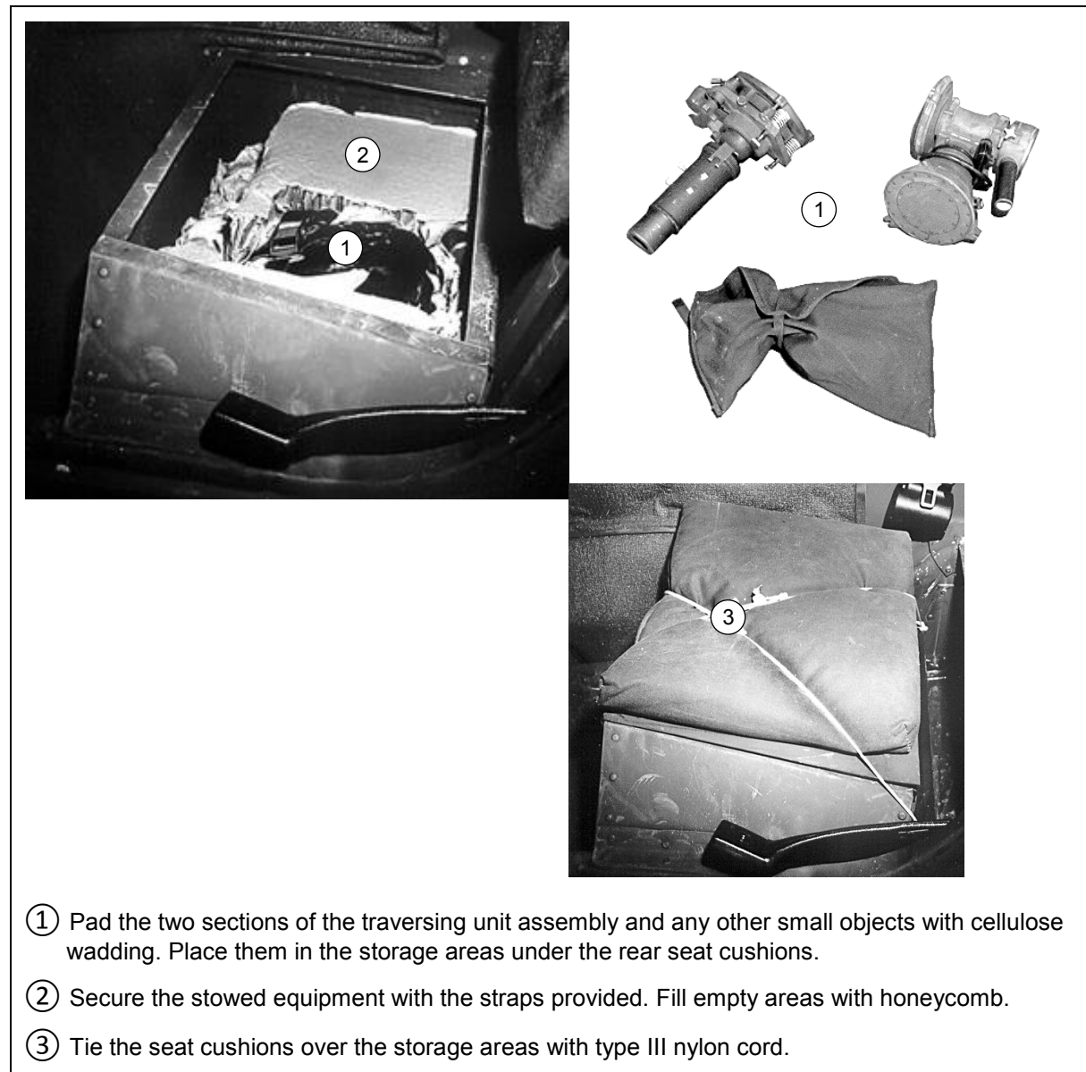
Figure 4-3. Ground/Vehicle Laser Locator Designator and Cab Accompanying Equipment Rigged in M966 Truck
