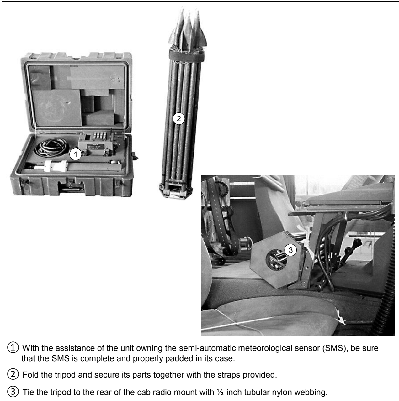
Figure 4-23. Rigging SMS in Cargo/Troop Carrier
