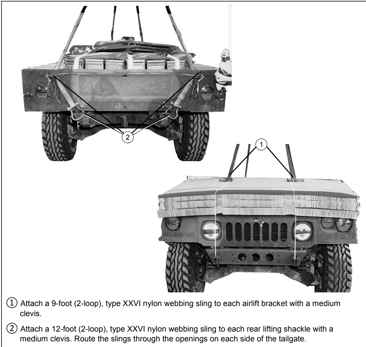
Figure 1-15. Lifting Slings Installed and Truck Positioned
