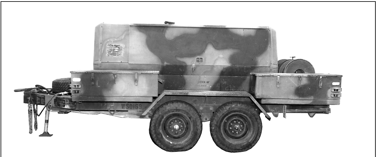
Figure 9-1. Ingersol-Rand Model, 250-CFM, Trailer-Mounted Air Compressor
