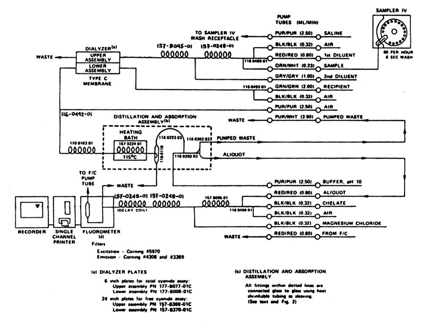
Figure 5-1. Flow diagram of manifold for assay of blood total CN- and plasma free CN-
