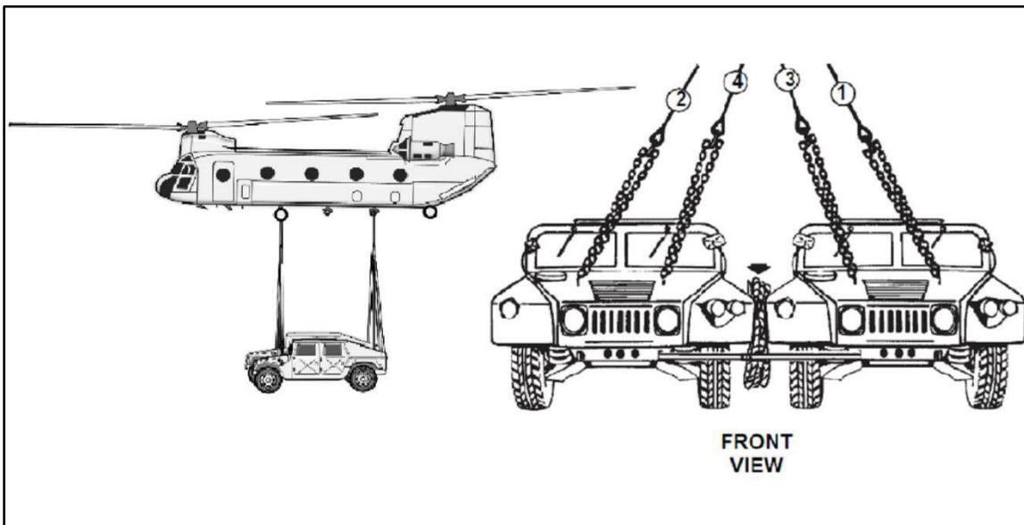
**Figure 5-4. Side-by-side (shotgun) sling load**
