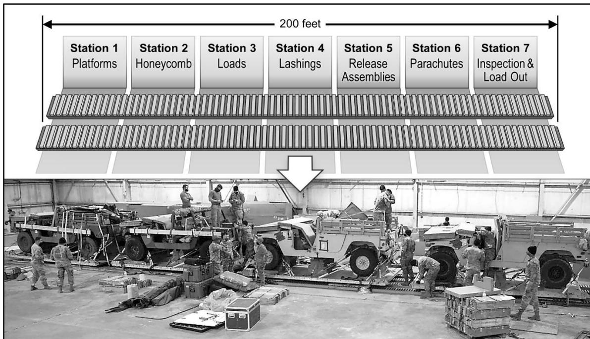
**Figure 4-11. Assembly line rigging layout**
