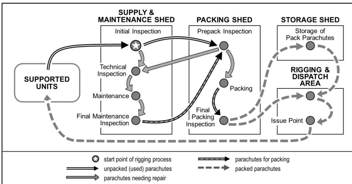
**Figure 4-7. Typical parachute packing process**
