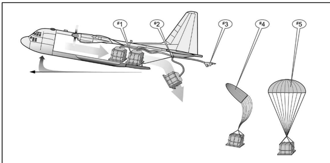
**Figure 4-4. Airdrop using the gravity airdrop method**
