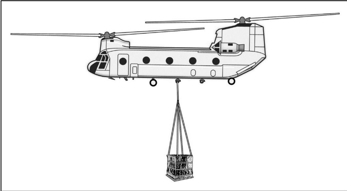
**Figure 5-1. Single-point sling load**
