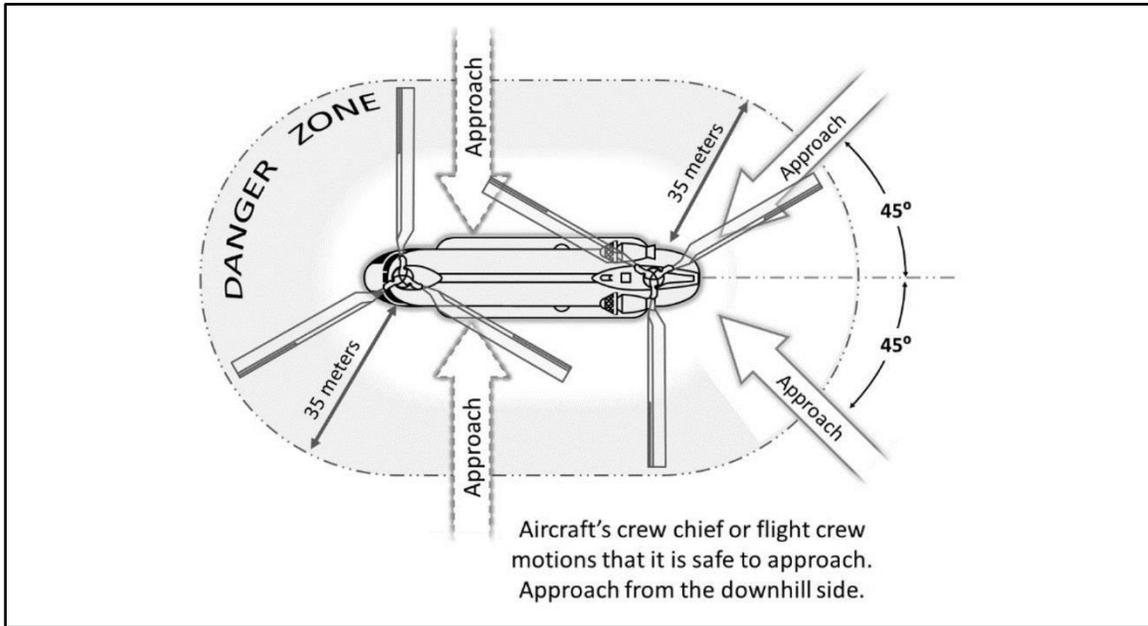
**Figure 3-2. Dual rotary-wing circle of safety**
