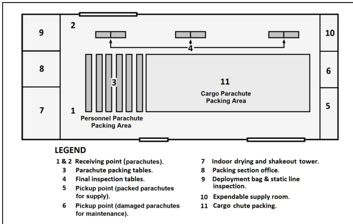
Figure 4-9. Suggested layout for a parachute packing shed
