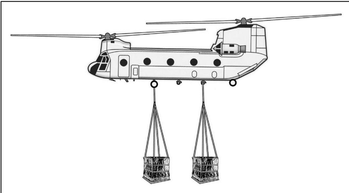
**Figure 5-2. Dual-point sling load**
