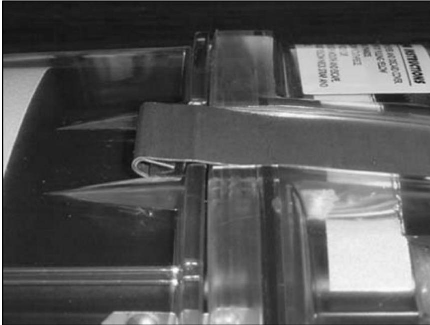
**Figure E-11. Hook latch assembly (incorrect band position)**
