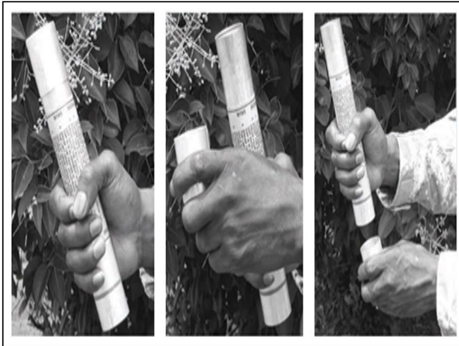
Figure E-2. Firing a signal flare
