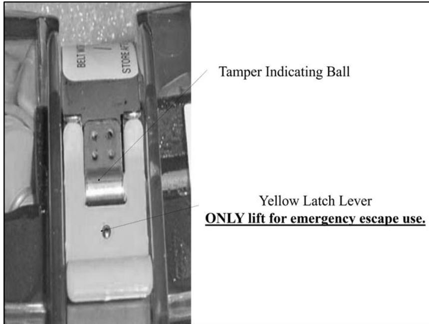
Figure E-6. How to inspect the M-20.2 EEBD
