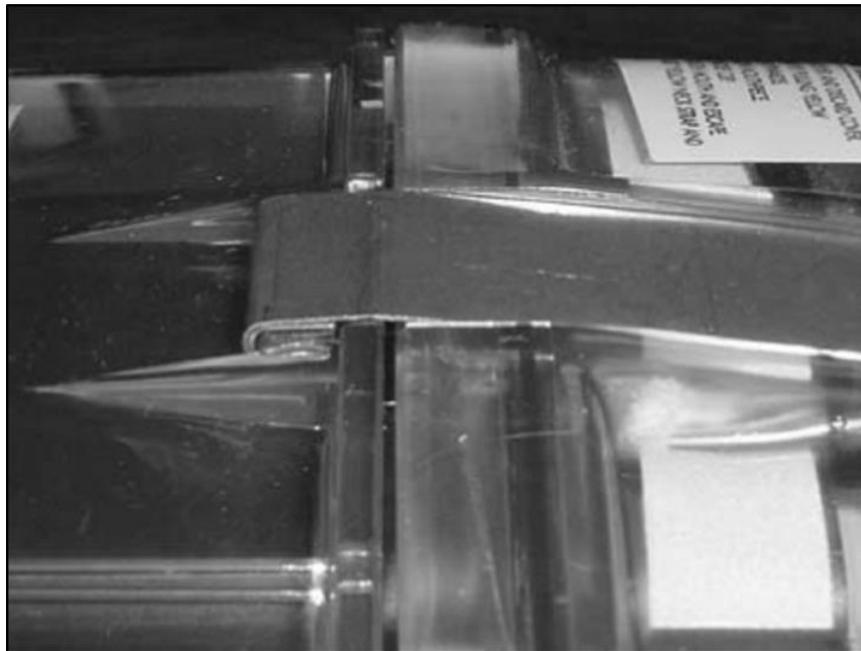
**Figure E-10. Hook latch assembly (correct band position)**
