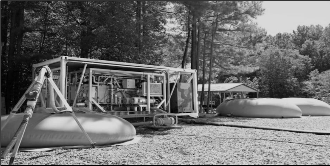
Figure A-2. Tactical water purification system
