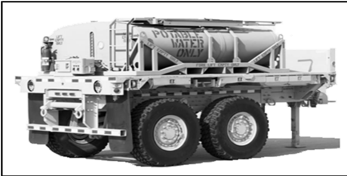
Figure A-13. Unit water pod system (Camel II)
