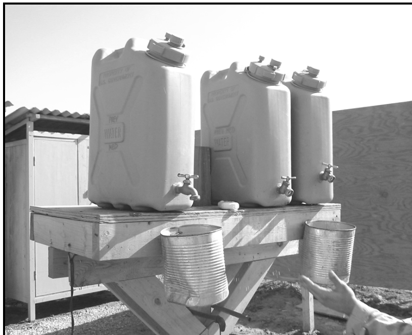
Figure 5-10. Improvised handwashing facility
