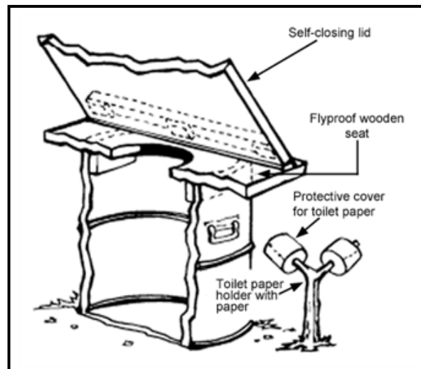
Figure 5-21. Single seat open-air burn-out latrine
