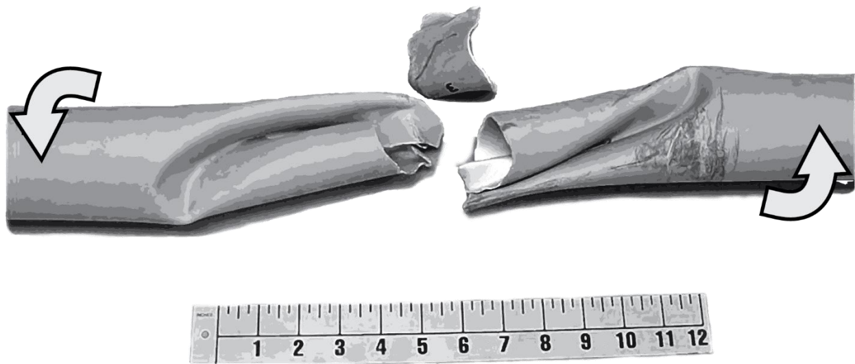
Figure F-6. Torsion load failure
