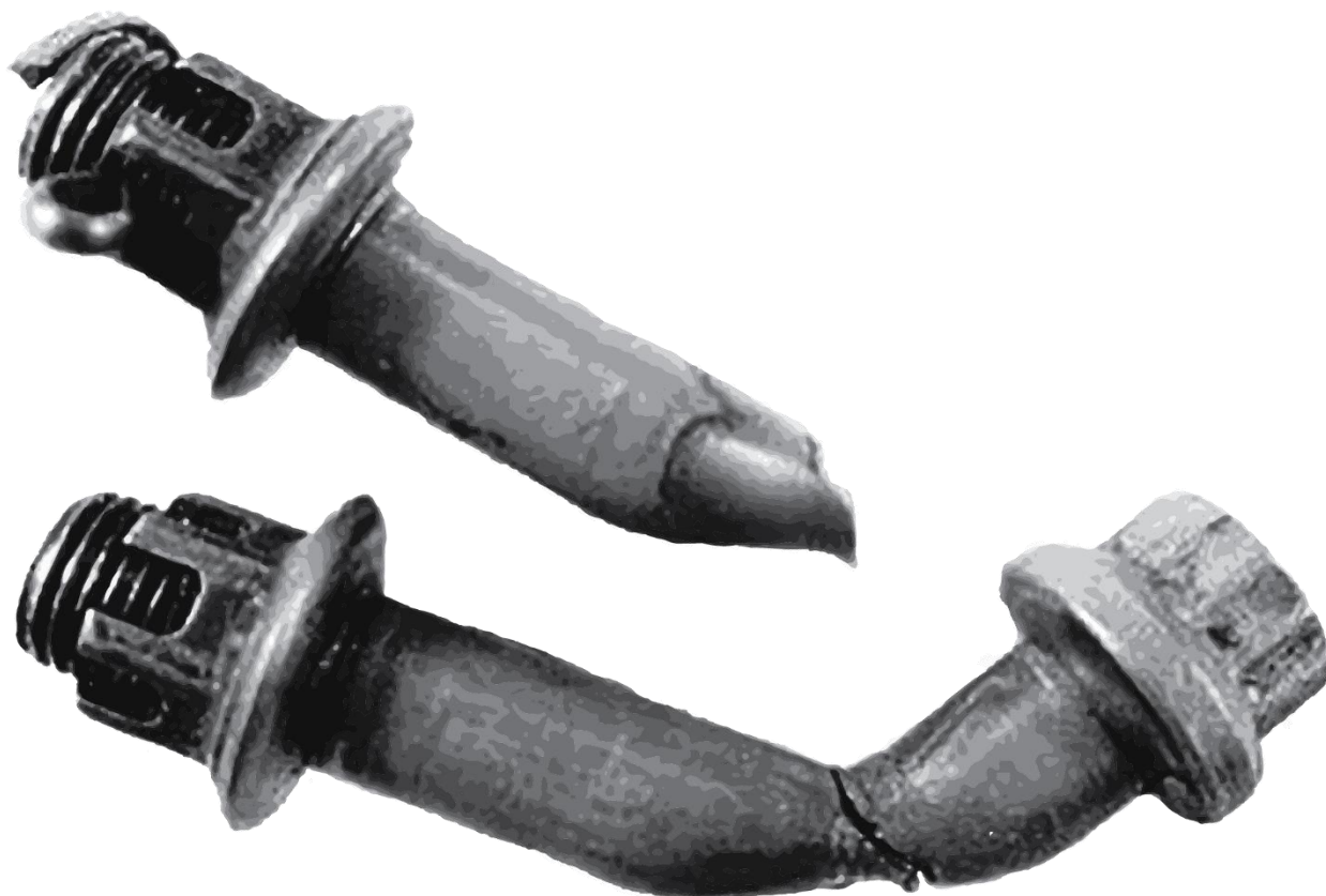
Figure F-7. Bending load failure
