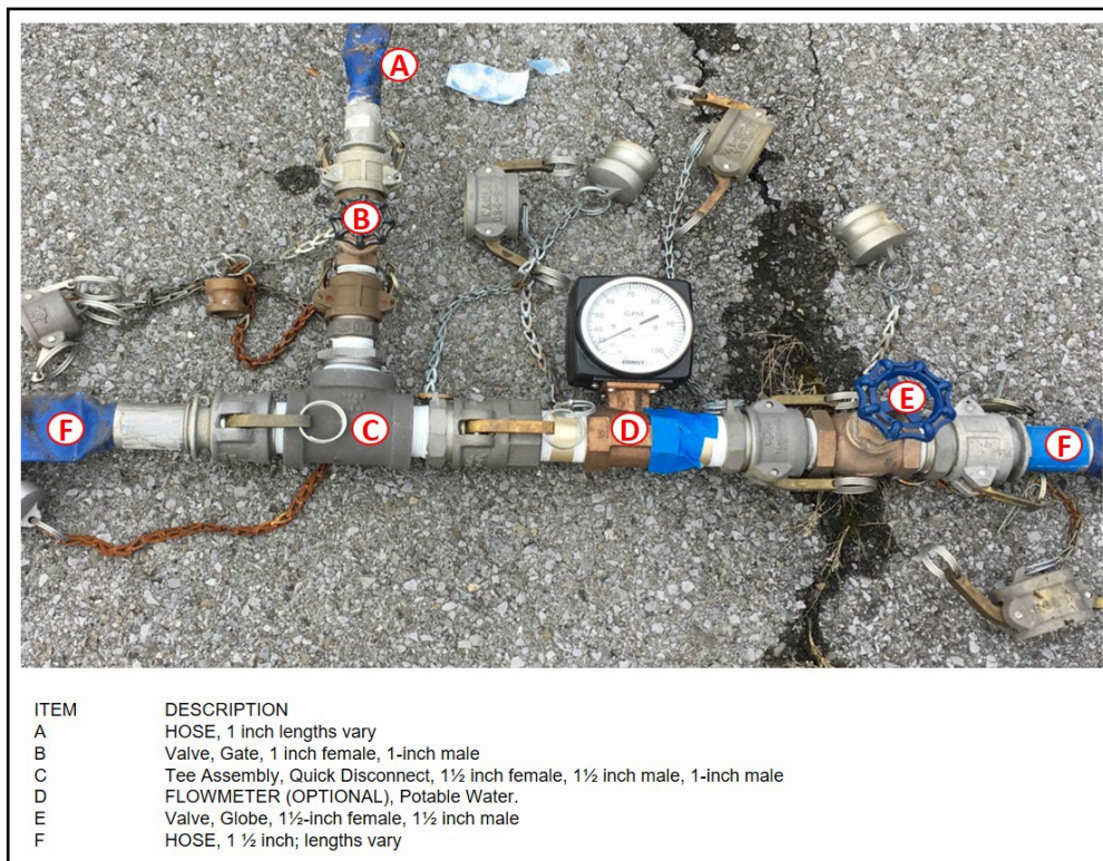
Figure 5-20. Fittings at the start side of a 1-in. loop
