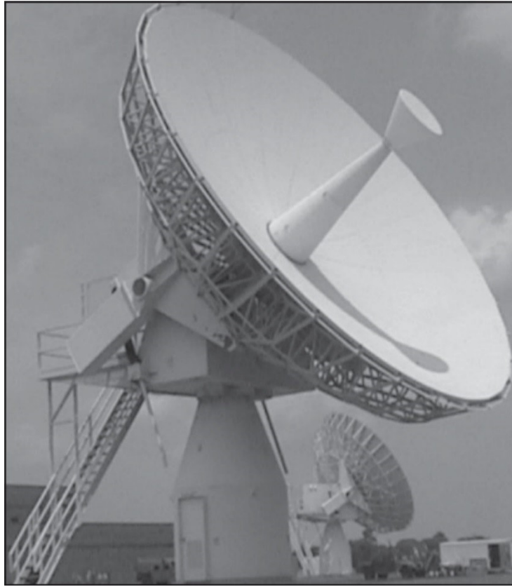
Figure A-4. AN/GSC-39(V1) terminal
