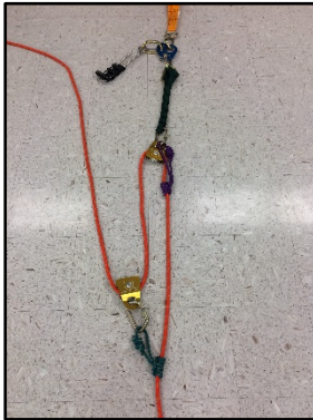
Figure 1-25. 3:1 mechanical advantage system
